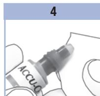
Remove the cap from the control solution bottle. Wipe the tip of the bottle with a tissue. Squeeze the bottle until a tiny drop forms at the tip.
