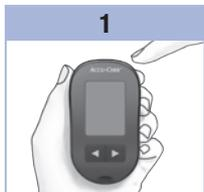
Press and release **⏻** (power/set button) to turn the meter on.
